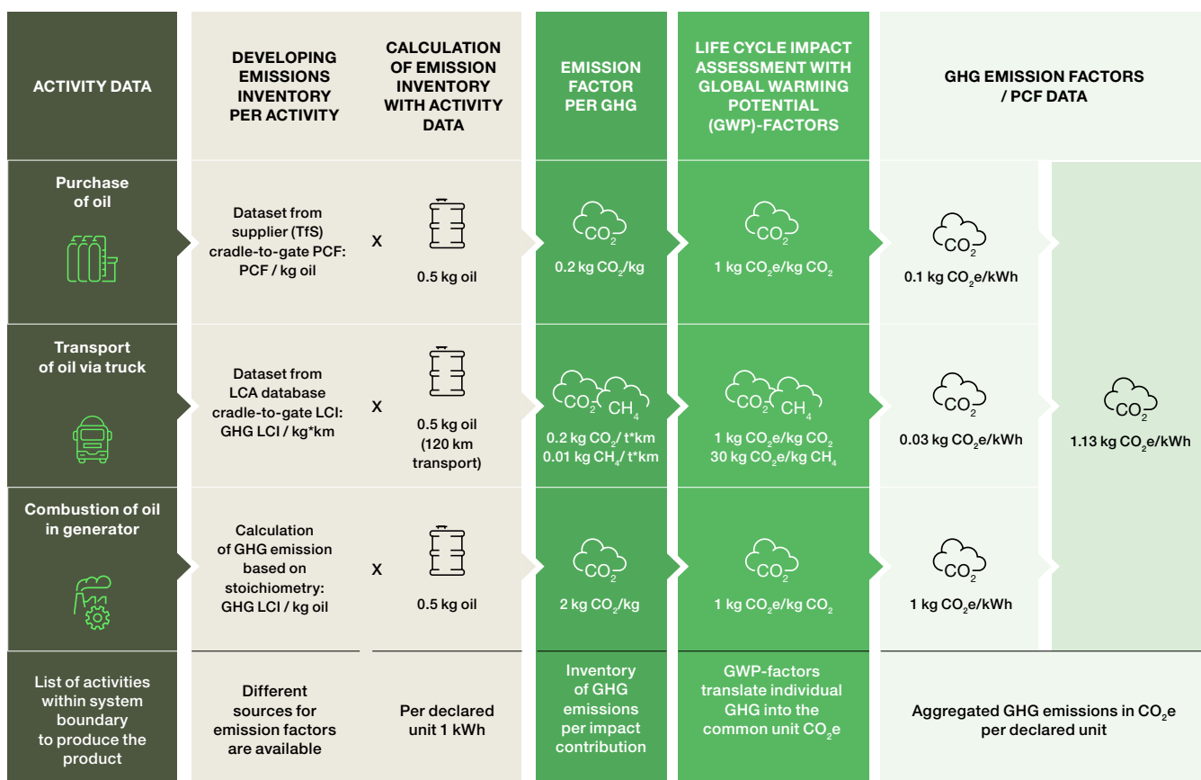
Figure 5.3 Types of data for PCF calculation on the example of production of 1 kWh of electricity
